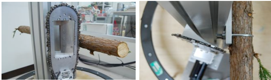
Figure 12. Chainsaw with circular slide guides for reducing thrust force
