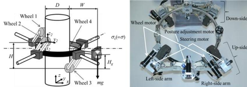
Fig. 1 Climbing robot equipped with four active wheel
