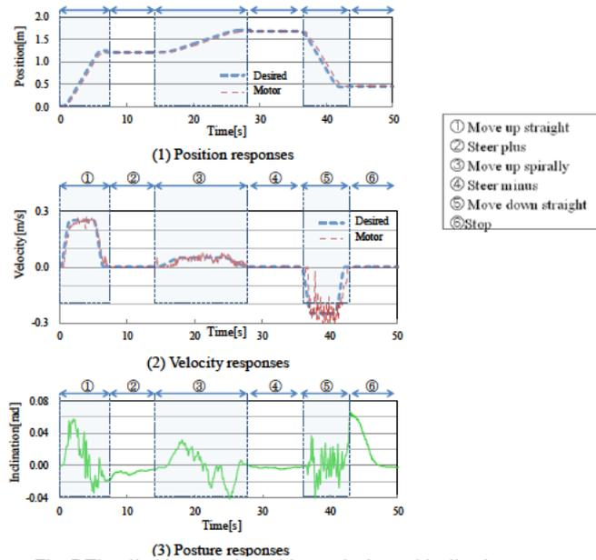
Fig. 7 The climbing robot's position, velocity and inclination responses to moving upward and downward (Left)
